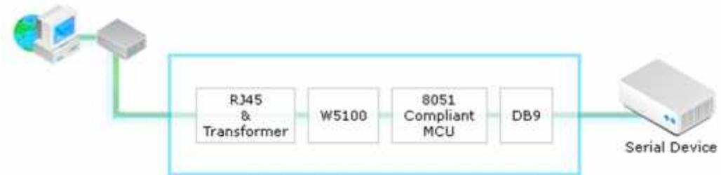
Gambar 2.5 Blok Diagram Board WIZ110SR
