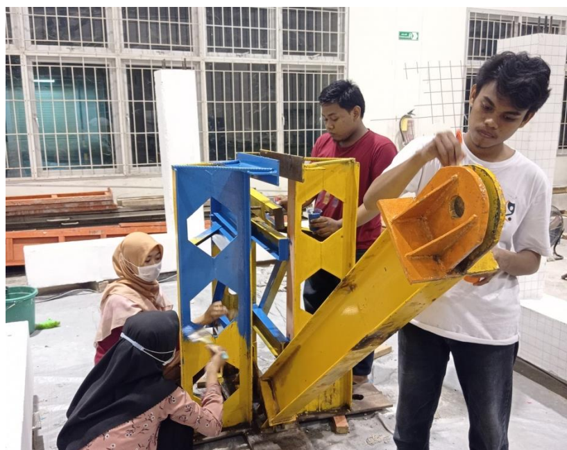
Pengecatan tiang support
