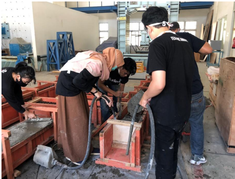
Pengecoran sampel beton BG-2
