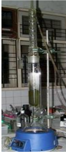
Gambar 5. Alat sokhlet (Lansida, 2012)
