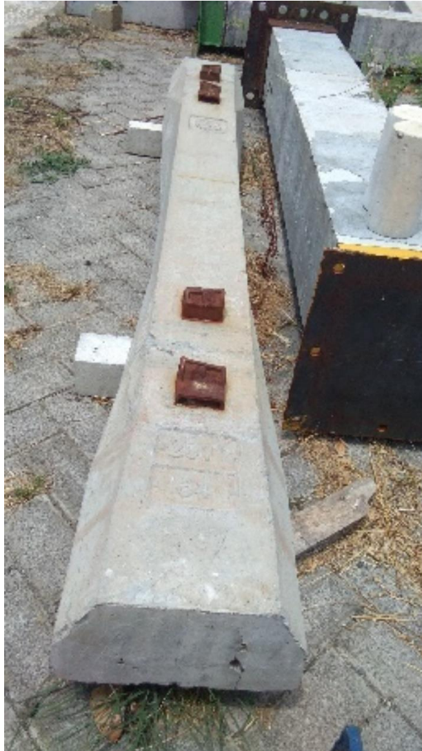
Gambar 17 Sleeper kereta api type BT25 S35 E68
