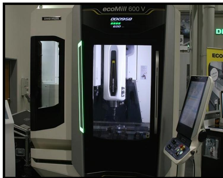
**Gambar 4 .** Mesin CNC Milling ecoMill 600 V (Journal DMG Mori, 2016)
