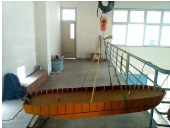
Gambar 20. Proses Penimbangan Model Kapal
