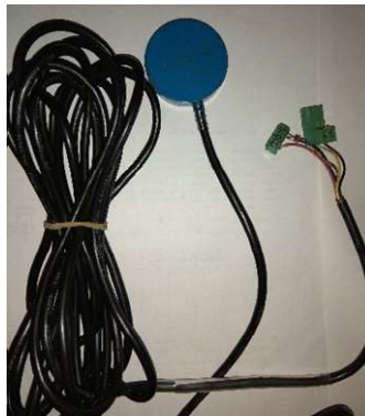
Gambar 2.7 Earth Pressure Cell Sensor
