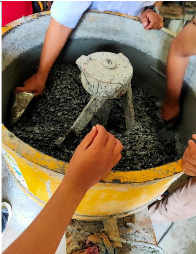
Mixing process of the Pervious Concrete Mixture using Laboratory Concrete Mixture.
