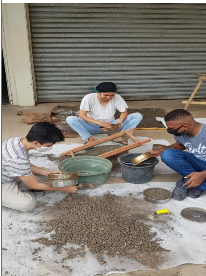
The Sieve analysis process of Nickel Slag and Crushed Stone as Coarse Aggregate for the Pervious Concrete.
