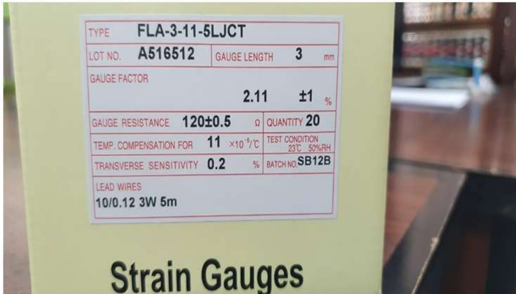
Gambar 40. Type Strain Gauge
