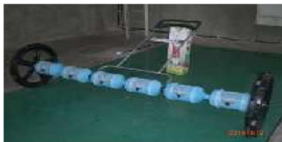
Gambar 2-5. Alat Tanam Benih Langsung Model Paddy Seeder Tipe Drum 12 Baris Sumber: Budiman, 2016
