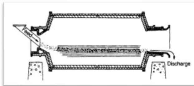
Gambar 2.2: Overflow Mill (thesimpleacre, 2013)
