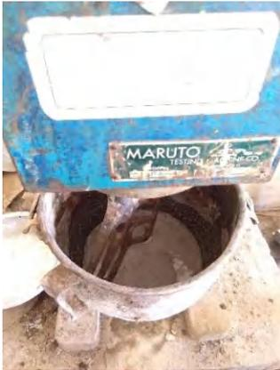
A blue and white mortar mixer machine with the brand name 'MARUTO' visible on its side. The mixing bowl is partially filled with mortar.                           | Pencampuran material dengan menggunakan mesin pengaduk Standar ASTM C 305 ( SNI 03-6825-2002 ) |
