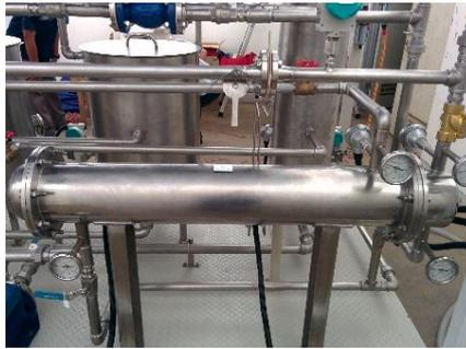
**Gambar 2.13** Heat Exchanger
