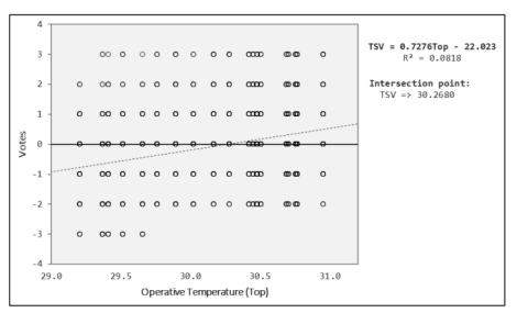
Figure 3. The Scatterplots and the Linier Regressions of the Operative Temperature (To) Versus the PMV During the Day
