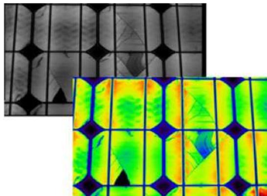
FIGURE 1. Cracks in the cell [10]
