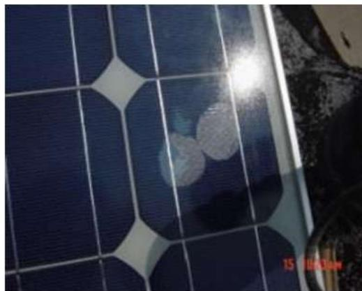
FIGURE 6. Partial shading of a PV module [7]
