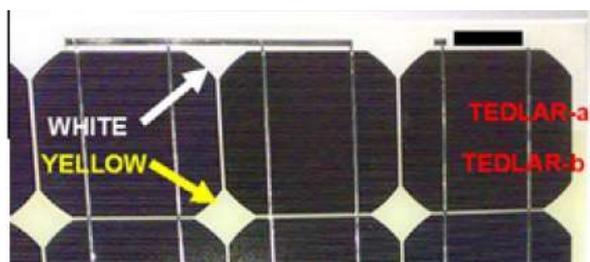
FIGURE 3. Discoloration of a PV module
