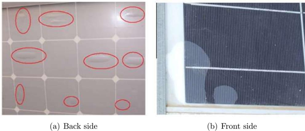
FIGURE 4. Bubbles on PV modules
