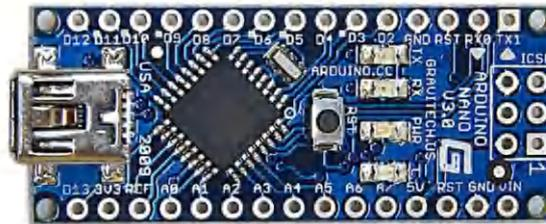
Gambar 1. Board Arduino Nano
