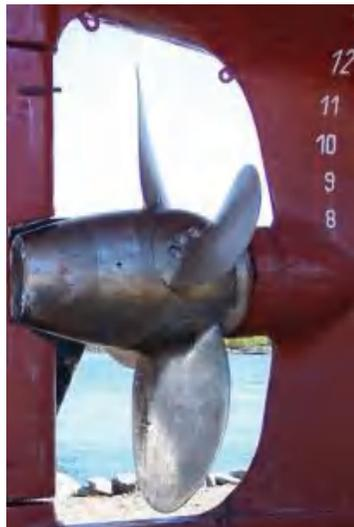
Gambar 1 Controllable Pitch Propeller
