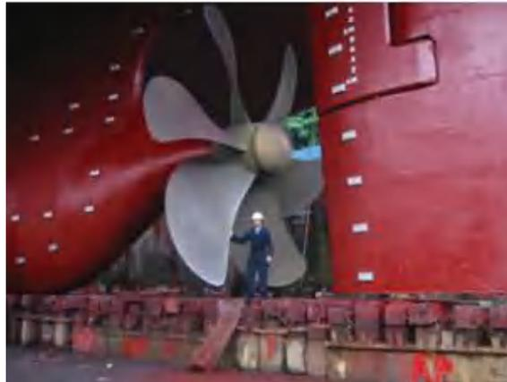
*Gambar 2 Fixed Pitch Propeller*
