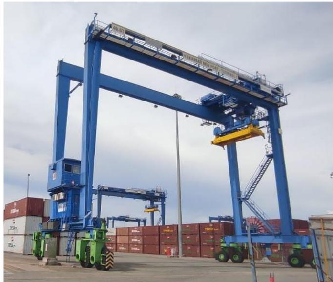
Gambar 2. 1 *Rubber Tyred Gantry Crane*
