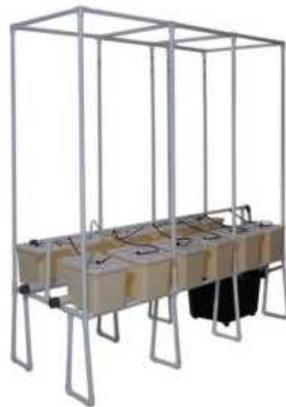
Gambar 18 instalasi dutch bucket
