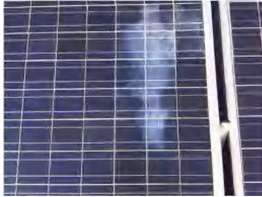
Gambar 6: Delaminasi (Sumber researchgate.net)
