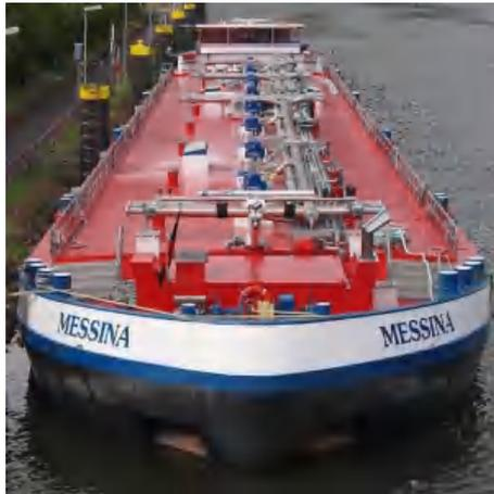
Gambar 2. 1 Liquid cargo Barge
