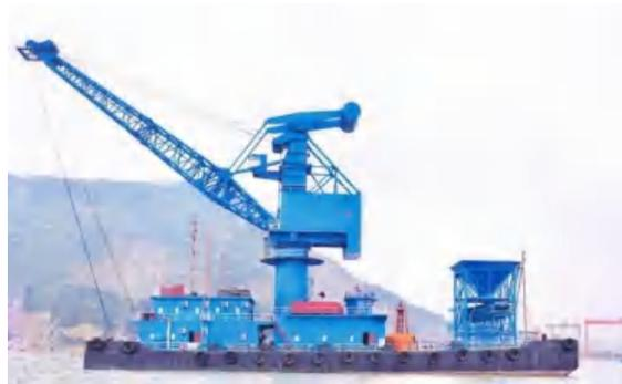
Gambar 2. 6 Crane Barge
