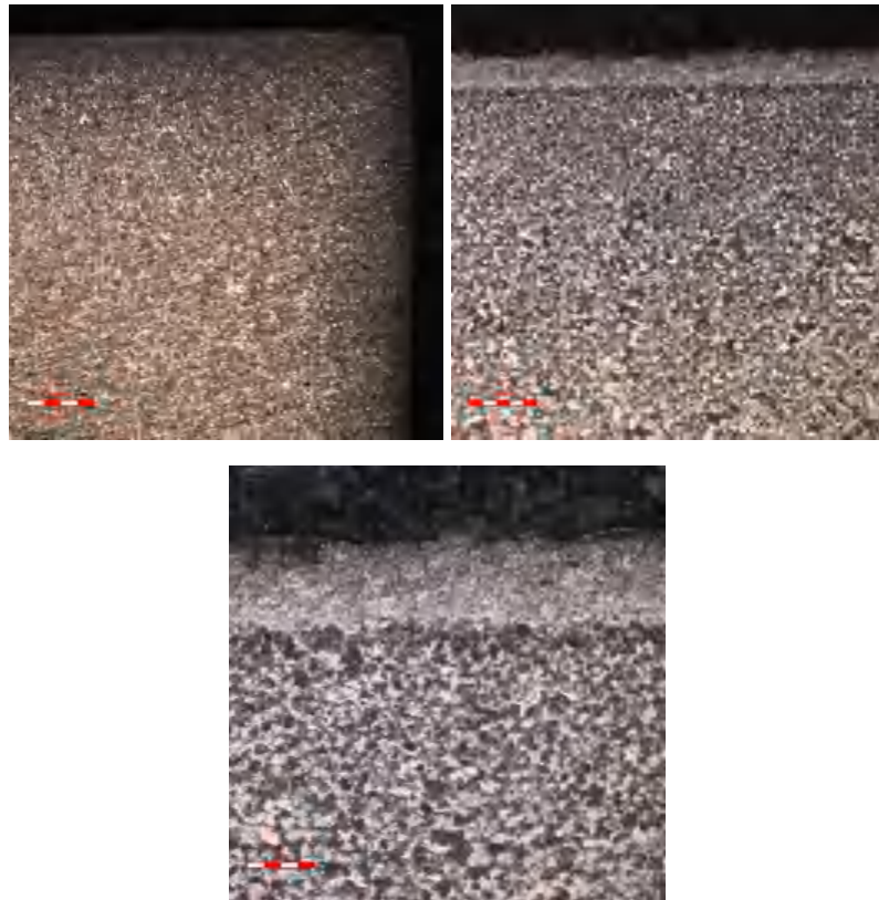
Microstructure galvanic treatment 1 Hari carburizing time 2 Jam
