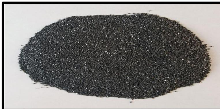
Gambar 3 *Silicon Carbide*
