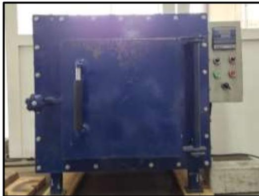
Gambar 19 *Furnace* (Max 1200°C)
