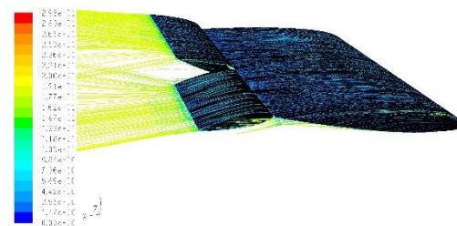
Sudut serang airfoil ( \alpha = -10^\circ ) dan U_0 = 20 m/s
