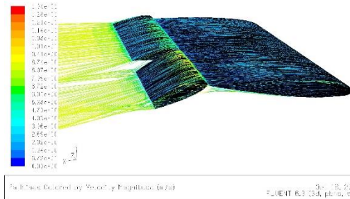
Sudut serang airfoil ( \alpha = -10^\circ ) dan U_0 = 9 \text{ m/s}
