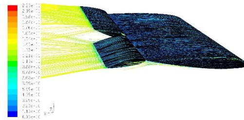
Sudut serang airfoil ( \alpha = -10^\circ ) dan U_0 = 15 m/s
