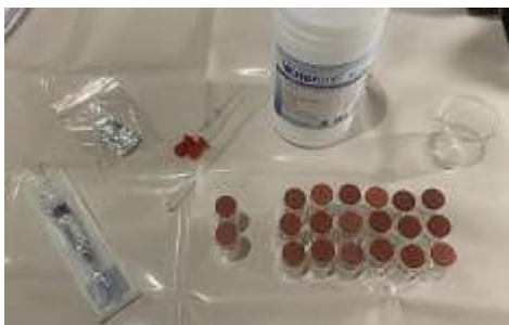
Preparation of mother liquor, dissolving GIC of group F8 with 1% DMSO
