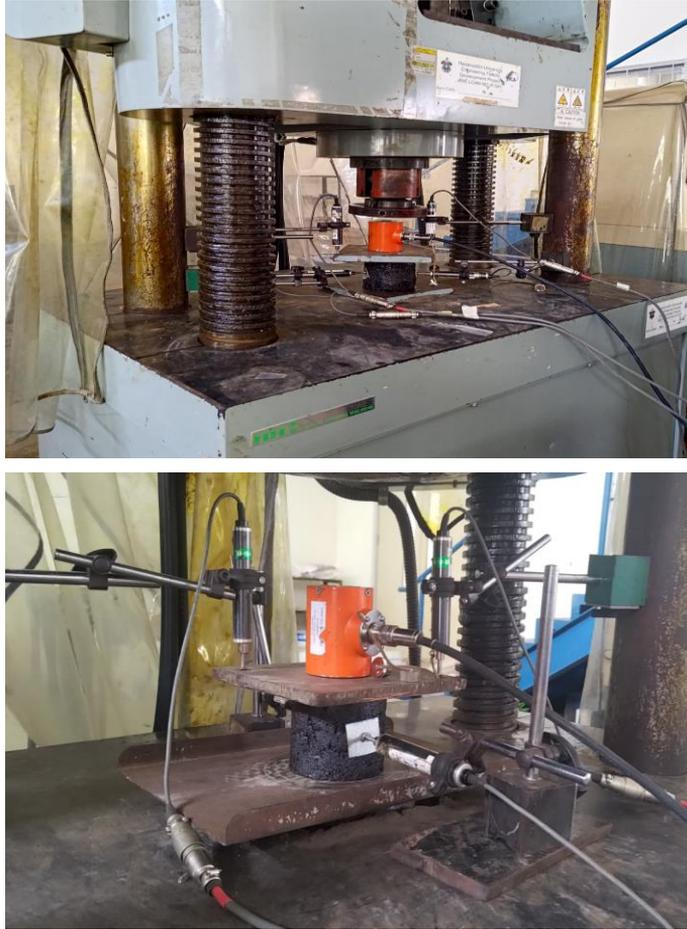
**Gambar 6.** Universal Testing Mechine
