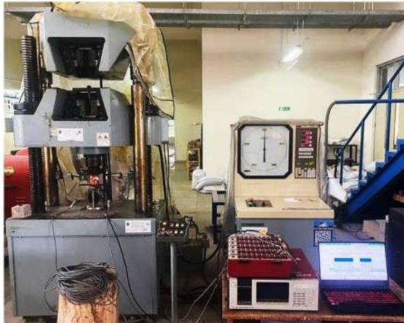
**Gambar 4.** Universal Testing Mechine
