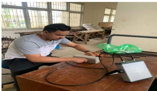
**Gambar 10.** Pengujian UPV Paving Block
