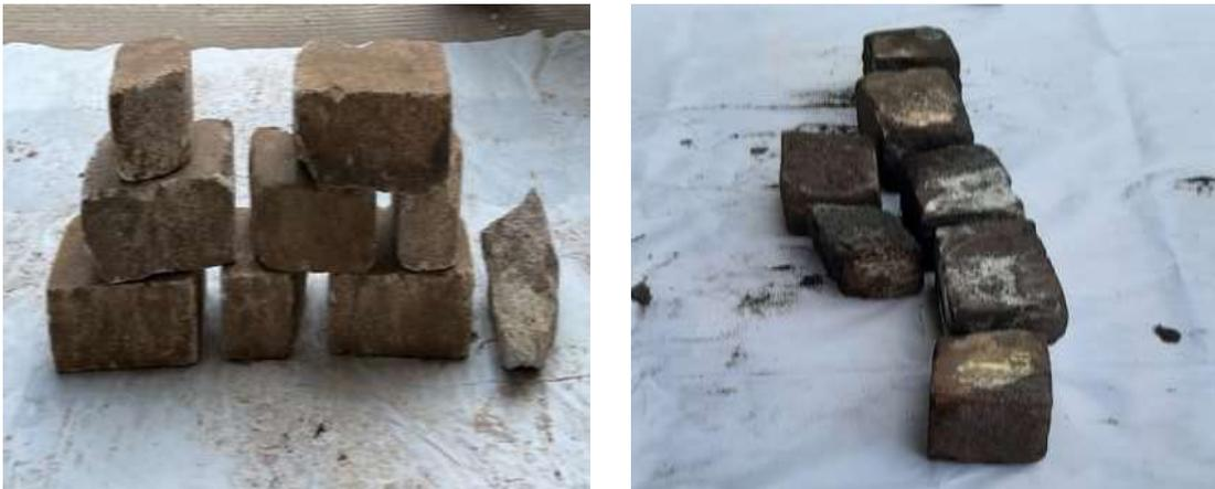
**Gambar 2** *Refractory Brick*
