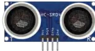
Gambar 2. 5 Sensor Ultrasonik HC-SR04
