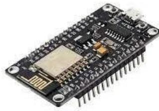
Gambar 7 NodeMCU
