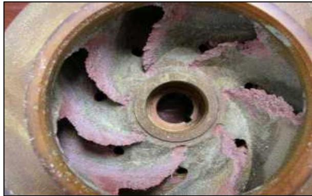
Gambar 6 Propeller Yang Mengalami Korosi Erosi
