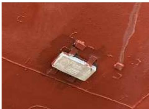
**Gambar 6.** *Quadpod zinc anode*
