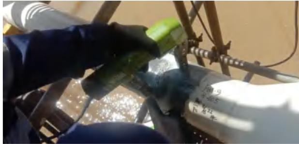
Gambar 2. 3 *Magnetic Particle Inspection*
