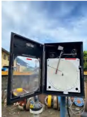
Gambar 2. 7 *Pressure recorder & temperature*
