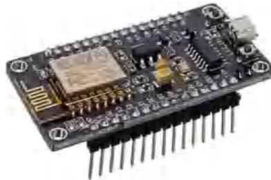
**Gambar 5.** NodeMCU ESP8226
