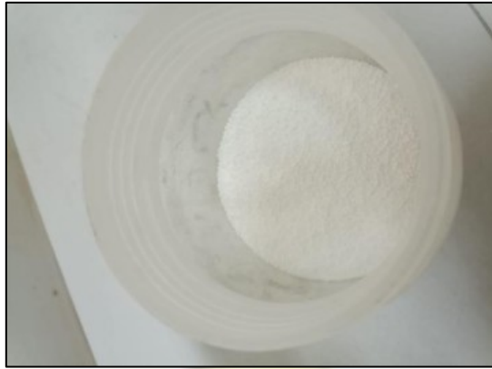
Lampiran Gambar 26 AN Prilled Defect Product
