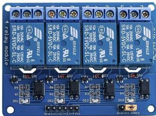
Gambar 2.5 Relay 4 Channel
