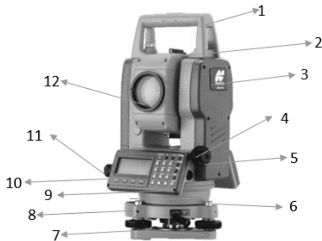
Gambar 2.5 Bagian-Bagian Total station (Uguy dan Pangalila, 2022)
