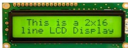
**Gambar 2.12** LCD 16x2 *Display* (Sumber: Andrianto & Darmawan, 2016)
