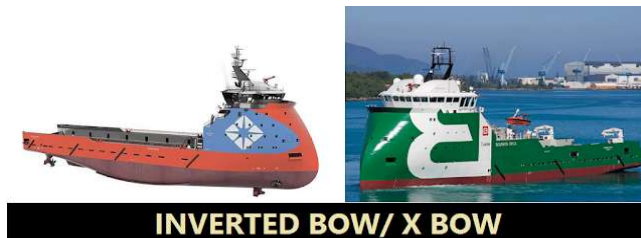
Gambar 8. Haluan kapal inverted bow
