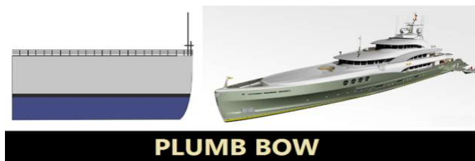
Gambar 1. Haluan kapal plumb bow/straight bow
