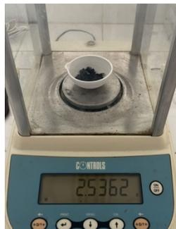
**Gambar 72. Penimbangan Sampel Briket Sebelum Masuk ke *Furnace***
