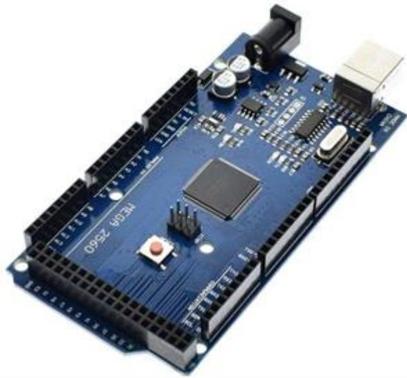
Gambar 4. Arduino Mega 2560
