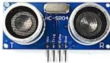
Gambar 11. Sensor ultrasonik HC-SR04
