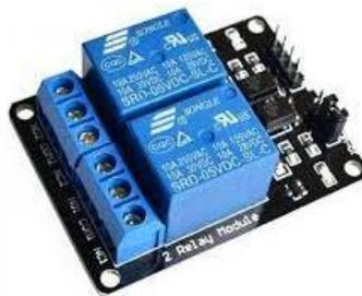
Gambar 15. Relay 2 Channel
