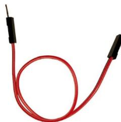
*Gambar 17 Kabel Jumper Male-to-Female*
