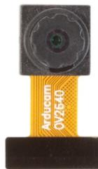
Gambar 2 Sensor Kamera OV2640
