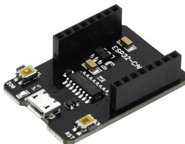
Gambar 3 ESP32-CAM Programmer Downloader
