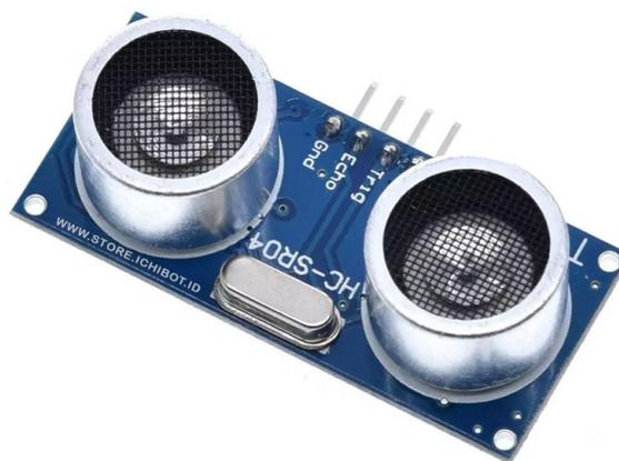
Gambar 6 Sensor Ultrasonik HC-SR04
