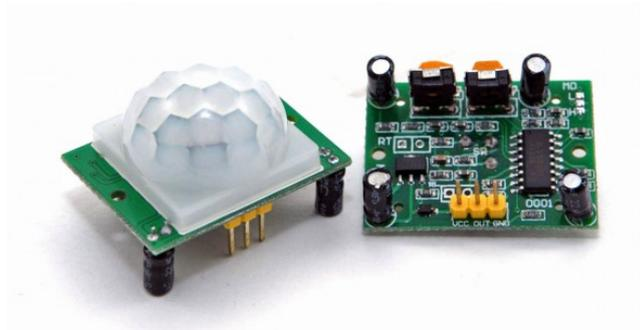
Gambar 4 Sensor PIR (*Passive Infrared Receiver*)
