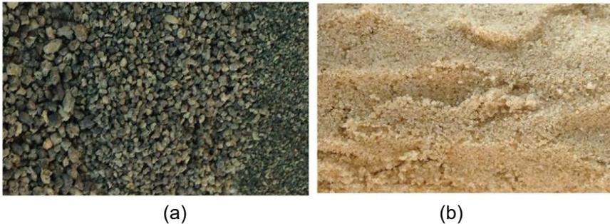
**Gambar 7** (a) Agregat FNS; (b) Pasir
