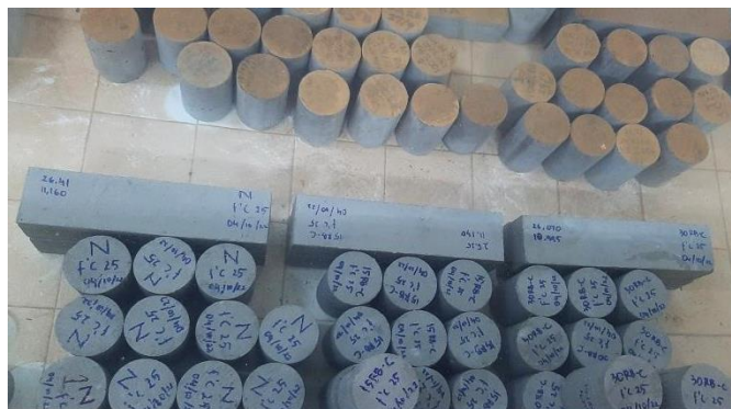
Gambar 12 Perawatan ( curing ) benda uji beton
