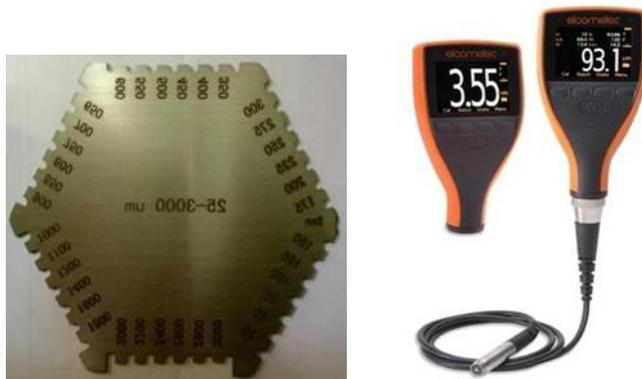
Gambar 6 *Comb gauge* dan *eletronik gauge*
