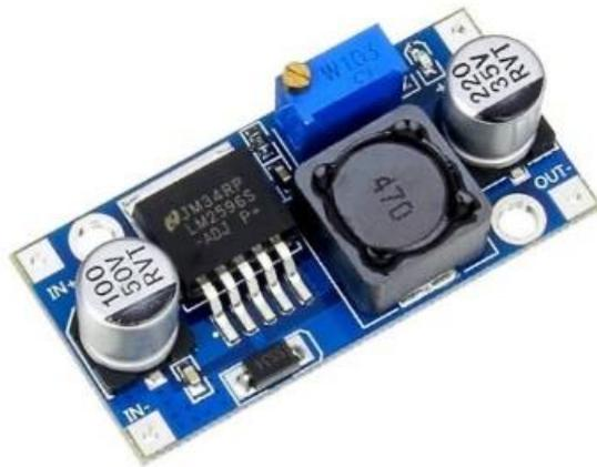
Gambar 9 Modul Step-Down LM2596
