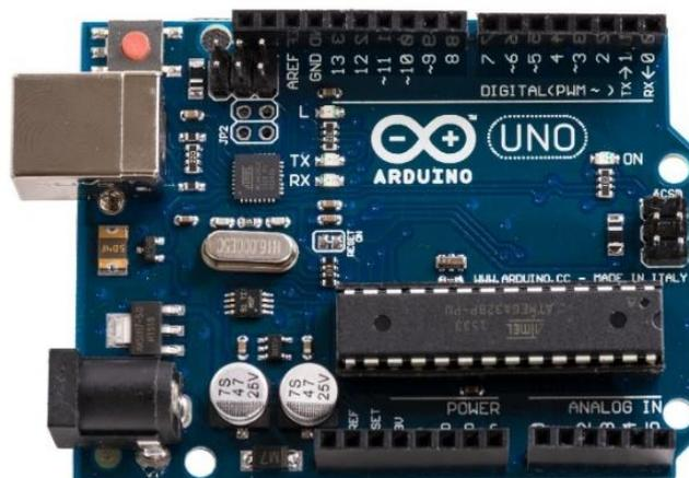
Gambar 4 Mikrokontroler Arduino Uno R3
