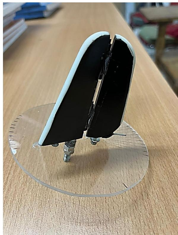
Gambar B. 2 Model spesimen pwngujian *smoke flow*
