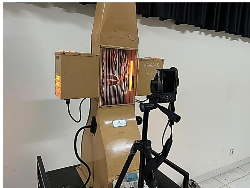
Gambar B. 4 Proses pengujian *smoke flow*
