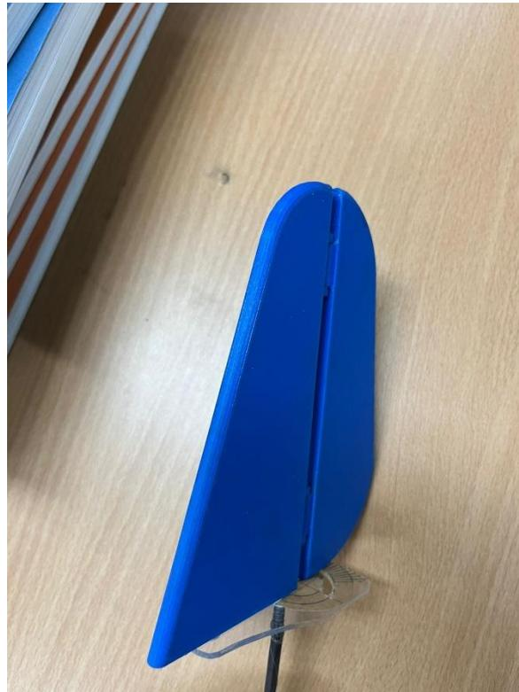
Gambar B. 1 Model spesimen pwngujian *wind tunnel*
