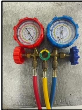
**Gambar 16** *Manifold Gauge*
