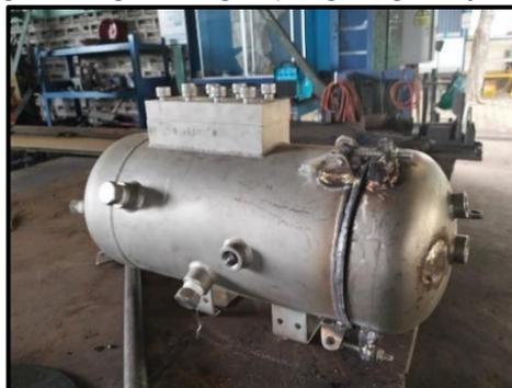
**Gambar 17** *Pressure Vessel*
