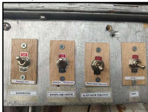
**Gambar 20** *Toggle Switch On/Off*
